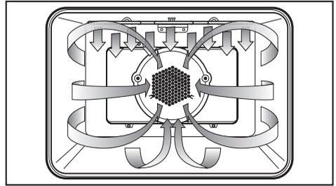
Always insert the grease filter over the convection fan in the back of the oven when using this function.
