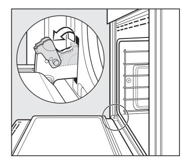
■ Slowly shut the door until the protruding clamps stop the movement. Pull the door upward. See illustration.
