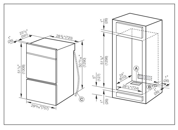
Vent (min. 24"<sup>2</sup> / 150 cm<sup>2</sup>) cut-out possible at rear or platform of cabinet
