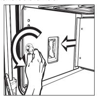
■ Use a coin or screwdriver to loosen the screw and remove the catalytic side panel from the oven.
