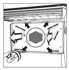
■ Loosen the screws in the back panel with a socket wrench and remove.
