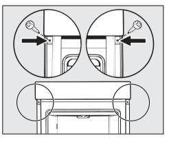
Open the oven door and using two screws secure it to the side walls of the housing unit through the holes in the oven trim.
