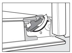
To release the locking clamps on the hinges turn them upwards as far as they will go until they are at an angle. See illustration. Then lift the door upwards as far as it will go.
