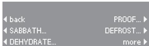
Dots after a function indicate a submenu.
