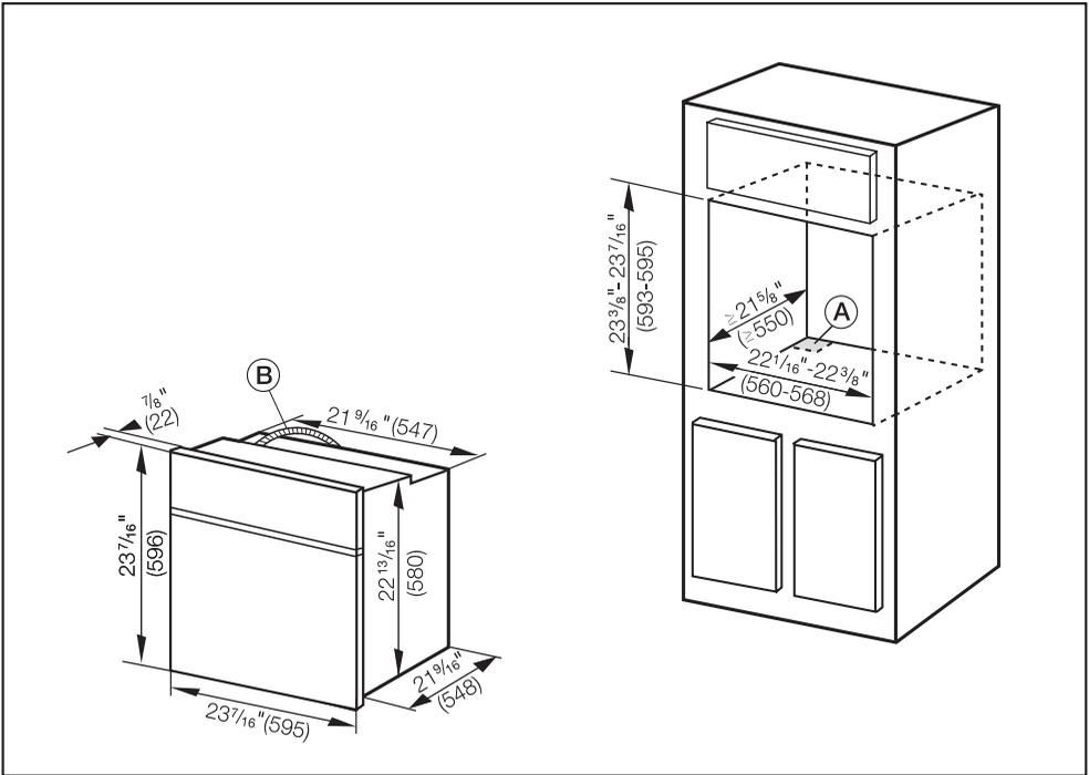
Ⓐ Cut-out for power cord (min.  $4^{\text{m}^2}$  /  $10\text{ cm}^2$ )
