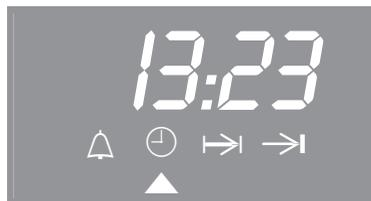
When the ▲ button is pressed, the **symbols for the clock/timer settings** that can be entered light up in the display.
