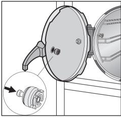
Insert the safety valve back into the inside of the door. Make sure that the seal fits correctly.
