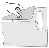
■ After cleaning, dry both parts of the insert thoroughly before replacing it in the water container. When replacing the insert (see illustration), guide it in at an angle ① and then push the side with the opening downwards ②.
