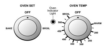
The **OVEN SET** knob determines the type of oven operation. Turn this knob to the desired setting. The oven will not operate if the **OVEN SET** knob is left in the OFF position.
