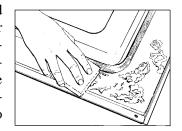
To prevent damage, do not clean or rub the gasket around the oven door. The gasket is designed to seal in heat during the clean cycle.
