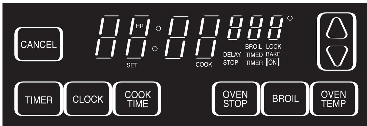
The electronic clock and oven control on your Maytag wall oven is used for the time-of-day clock, timer, bake, broil, and programmed operation functions. A beep will sound each time a function pad is pressed.
