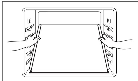
**To replace:** Fit the rear edge of oven bottom into the pin located at the center of the channel on the rear oven wall. Push toward the rear of the oven and lower oven bottom into place.
