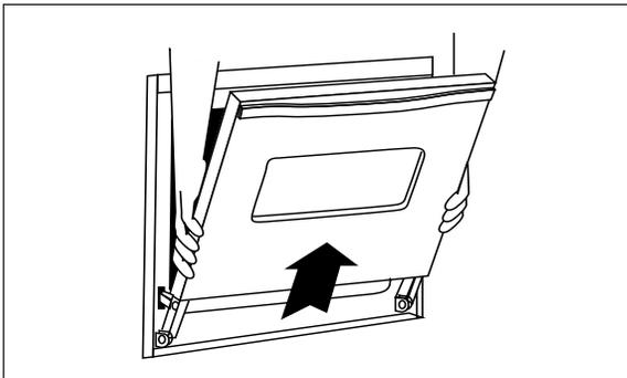
**Caution:** Hinge arms are spring mounted and will slam shut against the oven if accidentally hit. **Never place your hand or fingers between the hinges and the front oven frame.** You could be injured if the hinge snaps back.
