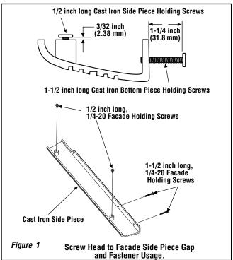
Step 3. Hook the two cast iron side pieces onto the fireplace side channels as shown in *Figure 2*. If the fit is too tight or loose, adjust the gap of the two holding screws. (See *Figure 1*.)
