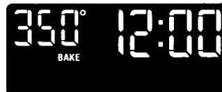
3. **To cook at a different temperature, use** the Temp pad(s). **Push ▲** to raise the temperature or **▼** to lower the temperature in 5°F increments. **Use** these pads until the desired temperature shows in the small display.
