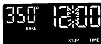
6. Use the Hour and Minute pads to set the desired stop time. Push the “up” (▲) or “down” (▼) pad(s) until the correct time shows in the display.
