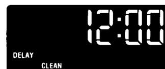
**Push** the Start/Enter pad. DELAY, CLEAN, and the time of day will light up in the display to show that the oven is programmed to start the Self-Cleaning cycle at a later time.
