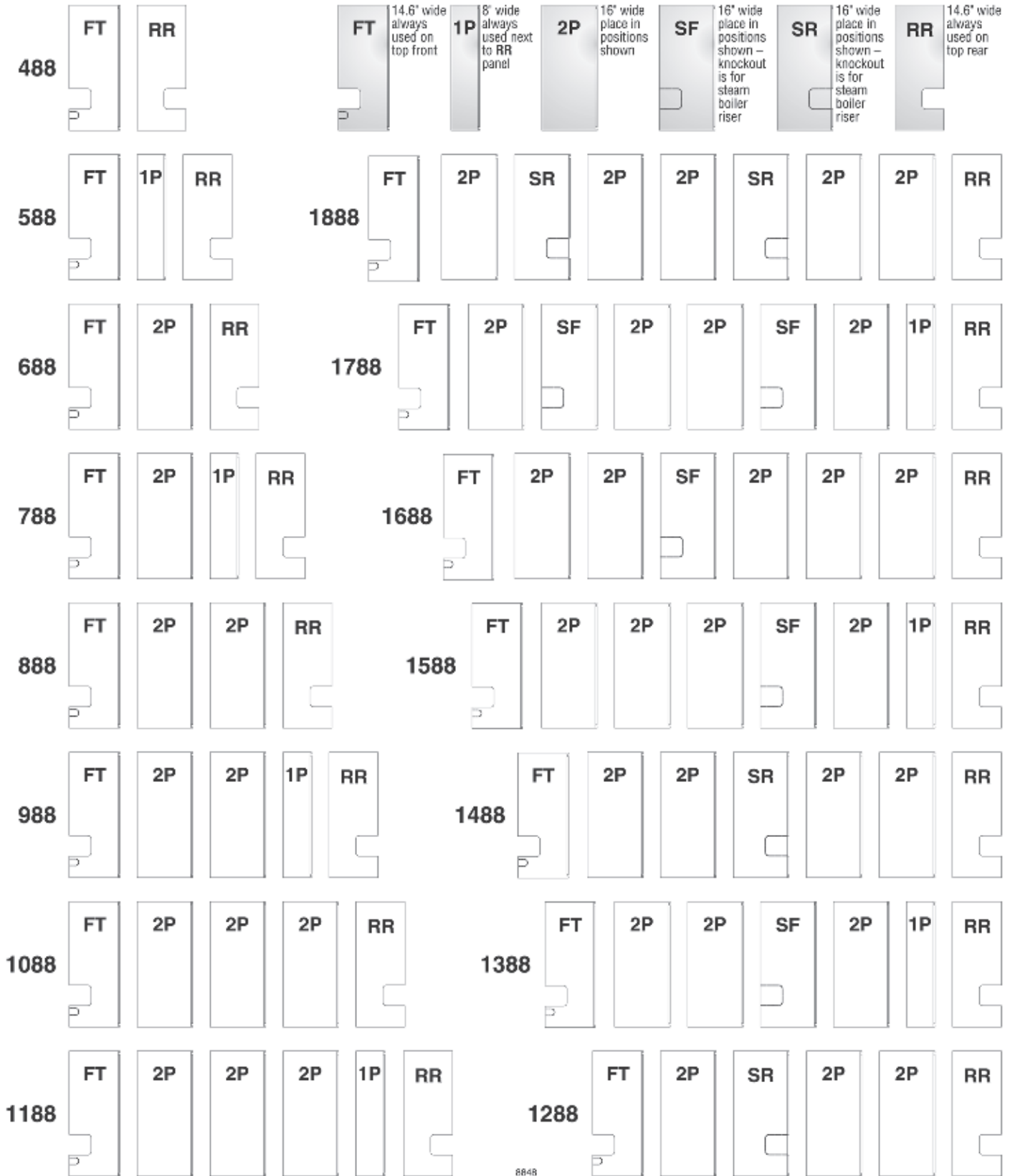
Figure 33 Jacket top panel placement
