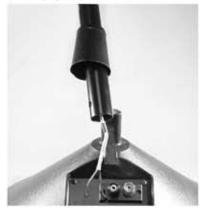
Slide second plastic cap up approx. 8" from bottom of the pipe.
