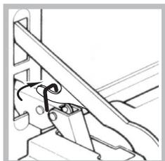
2. Lift up and turn the small levers located on the two hinges (*see diagram*).
