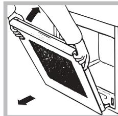
3. Grip the door on the two outer sides and close it approximately half way. Pull the door towards you, lifting it out of its slot (*see diagram*).
