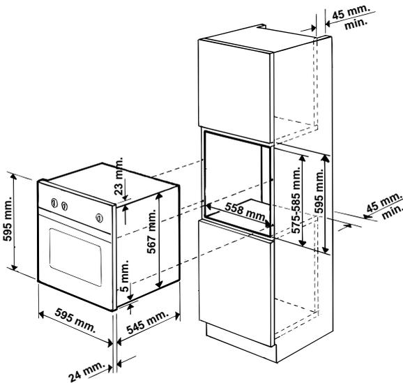
that it rests on two strips of wood is preferable. If the oven rests on a continuous, flat surface, there must be an aperture of at least 45 x 560 mm.
