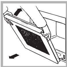
3. Grip the door on the two external sides and close it approximately half way. Then pull the door towards you lifting it out of its seat (*see diagram*). To replace the door, reverse this sequence.
