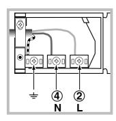
Voltage Frequency: 230 V-1+N 50Hz Fuse Section: 16A Supply cable: 3x1.5mm<sup>2</sup>
