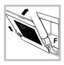
3. (With glass panel fitted to the inside of the door) Grip the door on the two external sides and close it approximately half way. Unlock the door by pressing on the clamps **F**, then pull the door towards you lifting it out of its seat (see diagram).
