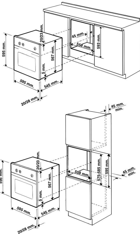
In order to ensure adequate ventilation, the back panel of the cabinet unit must be removed. Installing the oven so that it rests on two strips of wood is preferable. If the oven rests on a continuous, flat surface, there must be an aperture of at least 45x560 mm.
