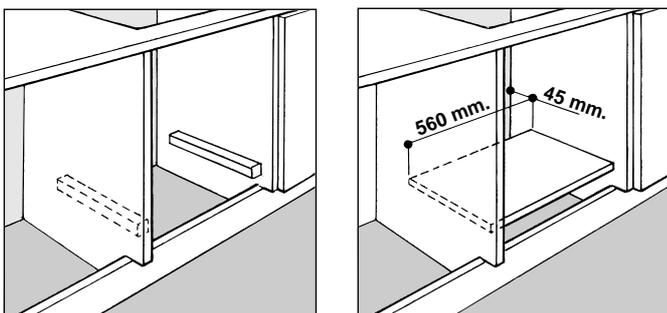
The panels of the adjacent cabinets must be made of heat-resistant material. In particular, cabinets with a veneer exterior must be assembled with glues which can withstand temperatures of up to 100 °C.
