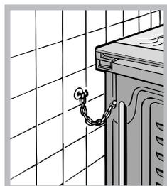
!Some models can have their gas connection inverted. It is important to make sure the safety chain is always situated on the side which corresponds to the hose holder (Fig. B).
