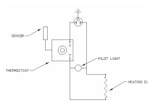
$480\ Volts\ /\ 1000\ Watts$   $20\ AMP/\ 480\text{-Volt}$  Grounding Plug NEMA 8-20P Not Provided
