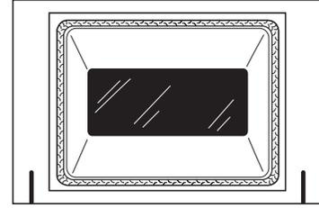
Do not rub or clean the door gasket—it has an extremely low resistance to abrasion.
