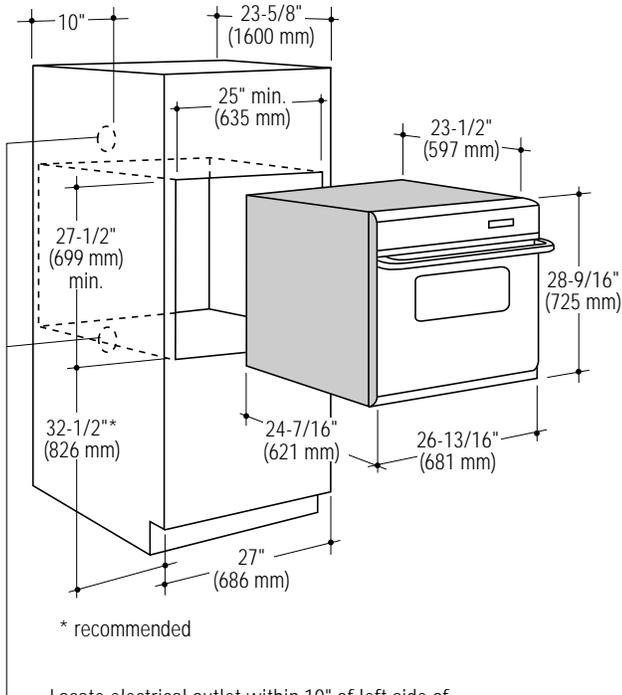
Locate electrical outlet within 10" of left side of opening 34" above cutout floor or 5" below cutout floor.
