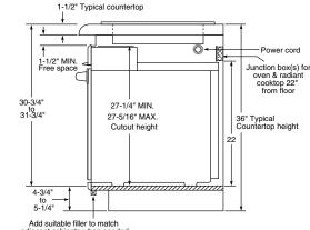
adjacent cabinets when needed to maintain toe kick alignment Side View
