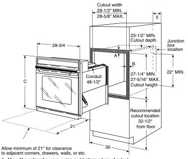
A=Allow 1" overlap of oven over top and bottom edges of cutout. B=Allow 11/16"-3/4" for overlap of oven over side edges of cutout. C=28-1/4" without trim and 28-3/4" with trim.
