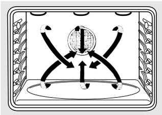
In a convection oven, a fan circulates hot air over, under and around the food.
