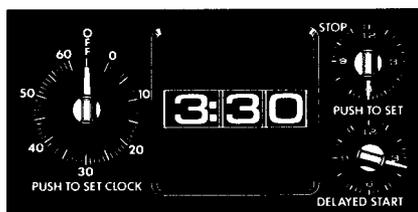
**Step 1:** To set Stop Time, push in knob on STOP dial and turn pointer to time you want oven to turn off; for example 6:00. The DELAYED START dial should beat the same position as the time of day on clock.
