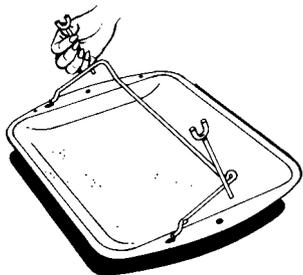
1. Assemble rotisserie. Insert curved ends of frame into large holes of broiler pan handles. Lock frame in place by fitting straight ends of support into holes in center handles.
