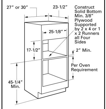
\* If you are replacing a GE/Monogram electric double oven with the combined installation of an Advantium 120 and a single oven, use the dimensions shown. The middle rail separating the two openings may need to be larger than the 2" minimum shown.
