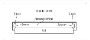
Place rail against cleats and flush with the outside edges of the cleats. Secure with wood screws. If the appearance panel is very narrow, cleats can be attached to the rail.
