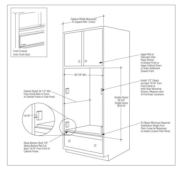
If you are using front framed cabinets with inset doors, these ovens can be installed flush with the front. In this installation the oven is completely recessed into the cabinet.
