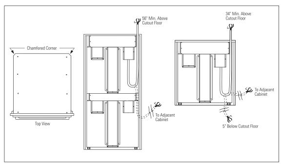
The back of the ovens have chamfered corners which provide a "chase" for the conduit when installing a junction box above or below the oven(s).
