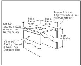
• Cut two pieces of 3/8" to 5/8" thick sheeting, to fit inside cabinet depth and available inside cabinet height. If there is no interference below the cutout, such as drawer runners, the sheeting can rest on the floor. Secure the sheeting strips or pieces to the cabinet walls with screws. Lay 2 x 4 or solid bottom on top of the sheeting and drive screws through the top and into the sheeting.
