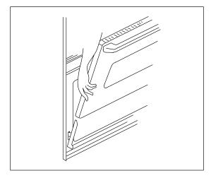
**Note**: The lower front trim is packed separately and should not be attached until the oven is installed and secured to the installation opening.
