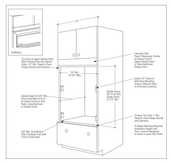
Use the information in this dimension drawing for typical frameless cabinets. The front face of the oven will be flush with cabinetry doors or drawers.
