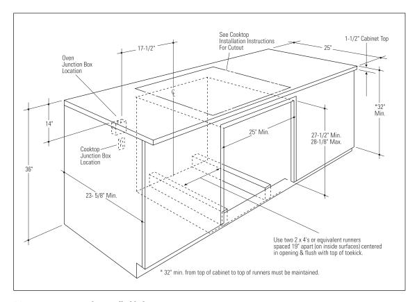
Monogram ovens can be installed below a countertop. The rough opening of the base cabinet should be:
