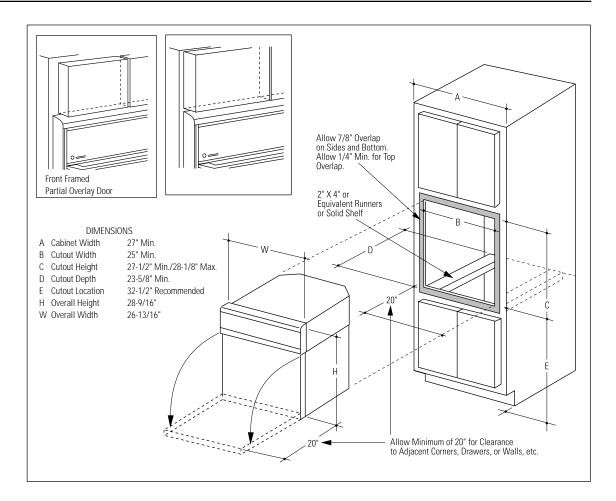
Use the information in this dimension drawing for typical framed cabinets. The front face of the oven will be flush with cabinetry doors or drawers.
