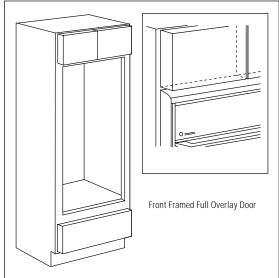
Monogram ovens are installed directly into a wall or wall oven cabinetry, 27" minimum width. The front surface of the ovens will be nearly flush with surrounding cabinetry. To obtain optimal appearance, cabinet cutouts must be exact. The examples shown here illustrate typical styles of 27" cabinets and oven fit. Installation instructions for each of these basic cabinetry styles are provided in this section.
