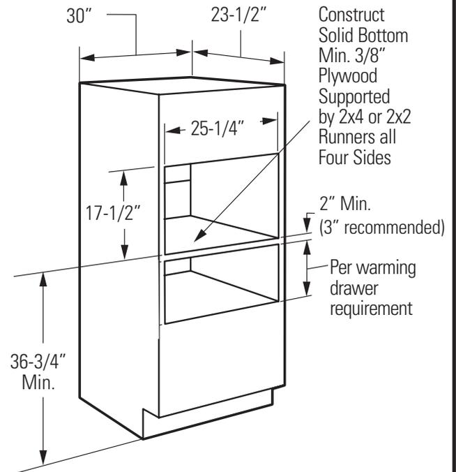
**NOTE:** Additional clearances between the cutouts may be required. Check to be sure the oven supports above the Warming Drawer location do not obstruct the required interior depth and height. See Warming Drawer installation instructions for details.
