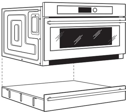
**NOTE:** The bottom of the oven side flanges will sit directly in front of the top of the storage drawer side flanges.
