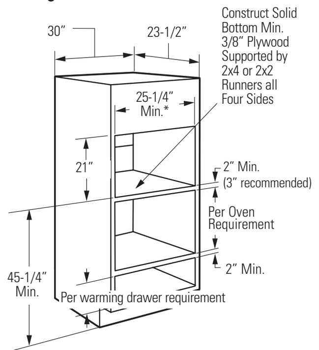
\* For existing cutouts, a maximum width of 28-1/2" is acceptable. If the opening is slightly wider, secure a furring strip on each side of the cutout for securing the oven.
