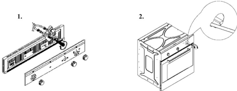
**IMPORTANT:** after having adjusted the burner, open and close the oven door to check that the flame remains lit at the minimum. If the flame goes out, adjust the by-pass setting.
