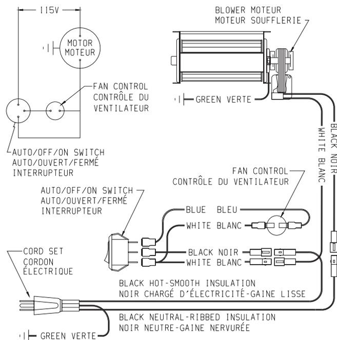
IF ANY OF THE ORIGINAL WIRE AS SUPPLIED WITH THIS UNIT MUST BE REPLACED, IT MUST BE REPLACED WITH NO. 18, 150°C WIRE OR ITS EQUIVALENT.
