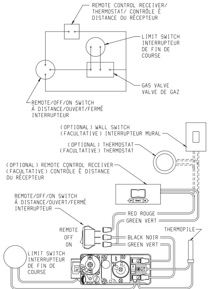
IF ANY OF THE ORIGINAL WIRE AS SUPPLIED WITH THIS UNIT MUST BE REPLACED, IT MUST BE REPLACED WITH NO. 18, 150°C WIRE OR ITS EQUIVALENT.
