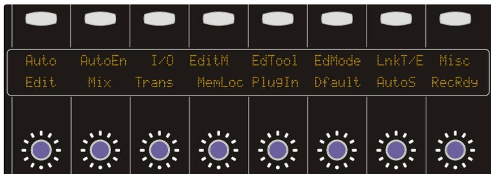
The two soft key sets are called **User 1** and **User 2**, and are activated by pressing the **User 1** or **User 2** switch, below the Nucleus logo in the centre section. The top row of the scribble strip display indicates the Mode switch function, the bottom row the V-Sel function. To return the Mode and V-Sel switches to their normal functions, deselect both **User 1** or **User 2** switches.
