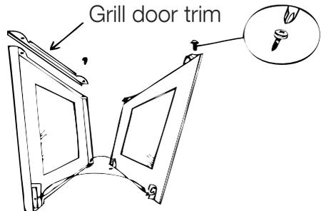
4. Holding the door and glass with one hand, gently pull towards you and slightly lift the door glass with the other hand to disengage the panel from the location point at the bottom of the door. Gently release the door to close it.
