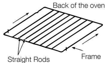
To remove a shelf slide the shelf towards you until the shelf stop is reached. Tilt shelf up at the front so that the stops clear the side supports. Lift shelf clear.
