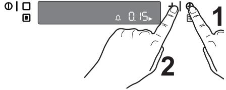
2. Touch control “+” to select the required time. The maximum time is 23 hours 59 minutes. After it is set, the minute minder waits 3 seconds and then starts running.
