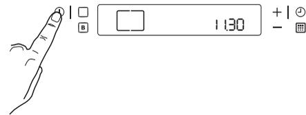
To switch off the oven, touch control
