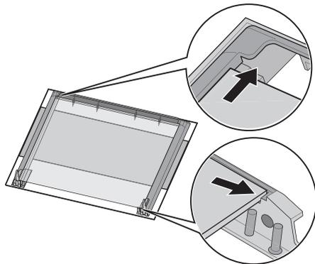
After the panes of glass have been reassembled in the oven door, perform the procedure described in point 8. in reverse to ensure they are locked.
