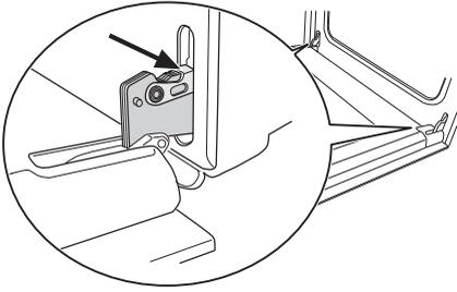
3. Lift and turn the levers on the two hinges
