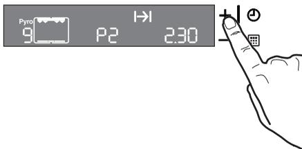
3. When you choose the desired pyrolytic function, **Pyro** will flash on the display waiting for confirmation to start the pyrolytic cleaning function.
