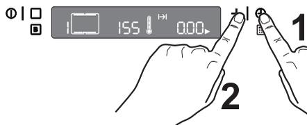
3. While the symbol ► is flashing, touch control “+” to select the required time. The maximum time is 23 hours 59 minutes. The programmer will wait 3 seconds and then start running.
