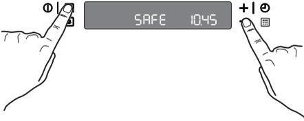
3. The oven is now locked. Neither oven functions nor temperatures can be selected.
