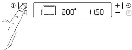
3. If the pre-set temperature is not suitable, touch control “—” or “+” to set the correct temperature. The temperature is adjusted in 5 degree steps.
