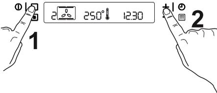
3. Set the temperature to 250°C by using the touch control “+”.
