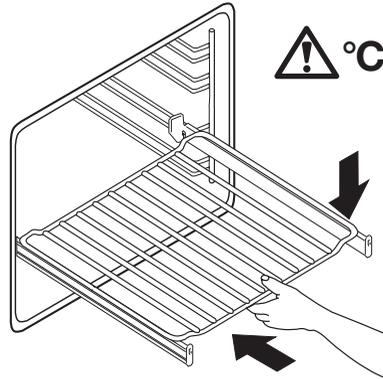
**!** **Warning!** Do not attempt to close the oven door if the telescopic shelf supports are not completely inside the oven. This could damage the door enamel and glass.
