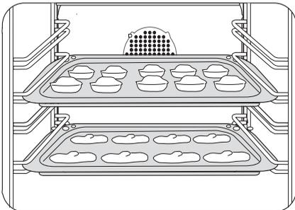
The constant air movement means no smell or taste is transferred between the different dishes. With fan cooking up to 2 trays of biscuits can be inserted at the same time. When baking or roasting on only one level it is recommended that you use the lower levels, so that you can see better. Fan cooking is particularly suitable for sterilising and drying mushrooms or fruit.
