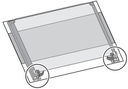
7. Release the locking system to remove the internal panes of glass
