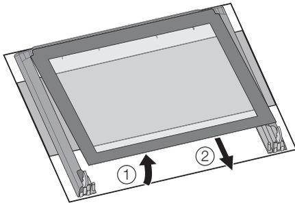
Clean the oven door with lukewarm water and a soft cloth. Do not use products such as scouring pads, steel wool, abrasive sponges or acids because they could damage the special heat-reflecting surface of the internal panes of glass.
