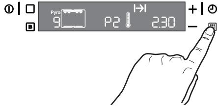
As soon as the oven heats up, the thermometer symbol rises slowly
