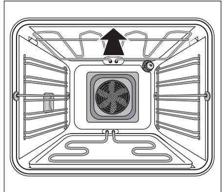
2. Rotate the fat trap to the left from the oven roof (see illustration).
