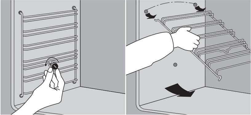
1. Undo the bolt (if necessary use a coin).
