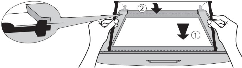
3. Lower the middle pane of glass (2) and slide it under the lower bracket to the stop.
