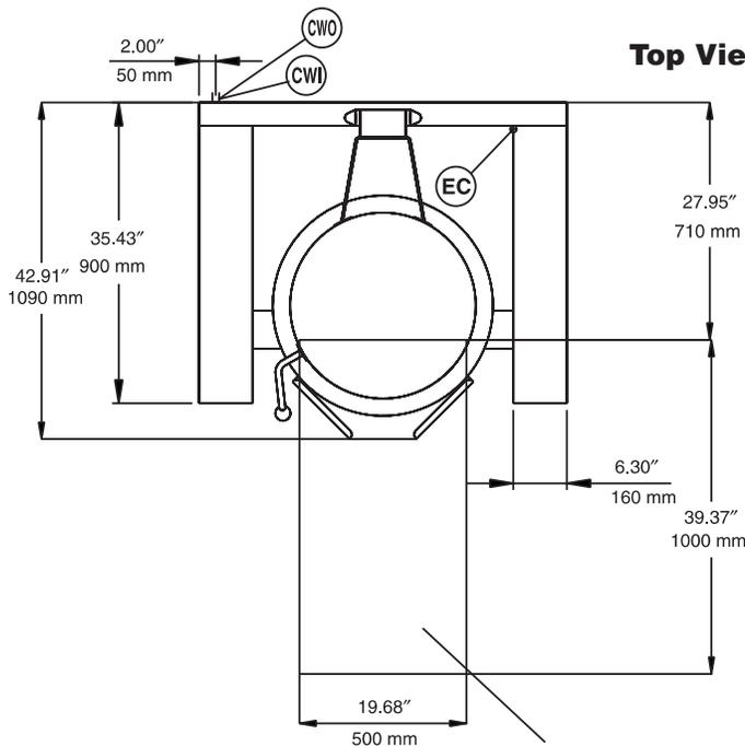
Maximum Pour Path/Suggested dimensions of drain trough
