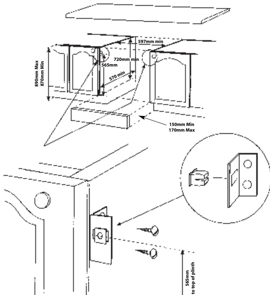
A minimum distance of 25mm should be maintained between the front face of the cabinet side and the front face of the plinth.
