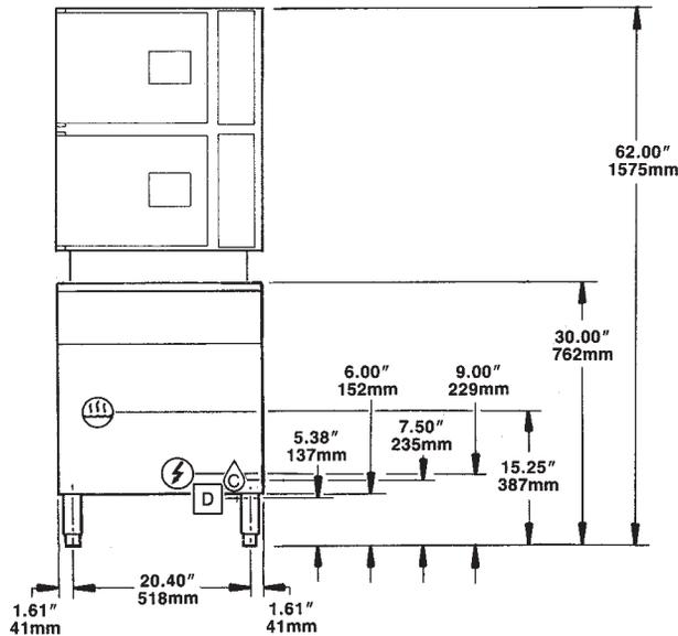
**NOTE:** When ordering optional reverse door openings: Control Panel, door openings, and cooking compartments are opposite that shown. Required clearance on left side, when ordered with reverse door openings, is 12.00" if adjoining wall or equipment is over 30.00" high.
