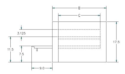
BK-18 & 22 HAVE ONLY ONE STANDARD STEEL BAKING DECK (LOWER SHELF) OR OPTIONAL CERAMIC HEARTH BAKE DECK AS PO-18/22. OVENS ARE STACKABLE.
