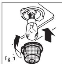
**IMPORTANT: Never use screwdrivers or other utensils to remove the light cover. This could damage the enamel of the oven or the lamp holder. Remove only by hand.**
