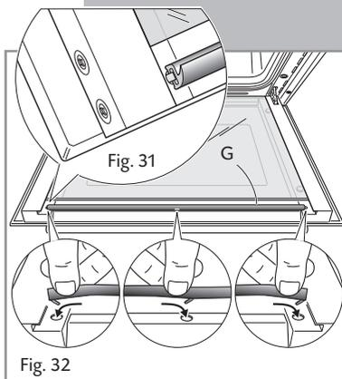
The oven door has a sealed gasket in the top part.
