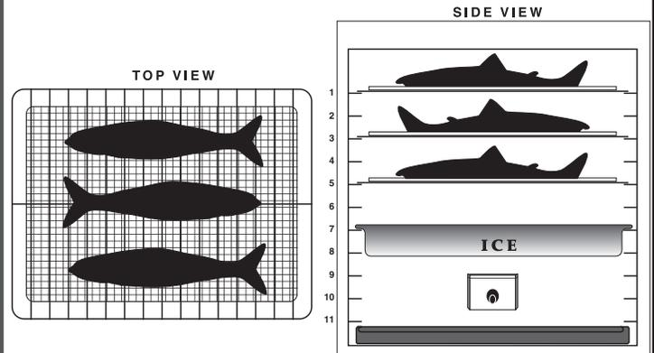
Insert probe of thermocouple thermometer into the center of the middle salmon fillet located in the top shelf position or central shelf position when smoking a full load. To maintain proper color, the internal temperature of the salmon must not exceed 77°F (25°C). For this reason, it is important to begin the smoking process with the oven at room temperature.
