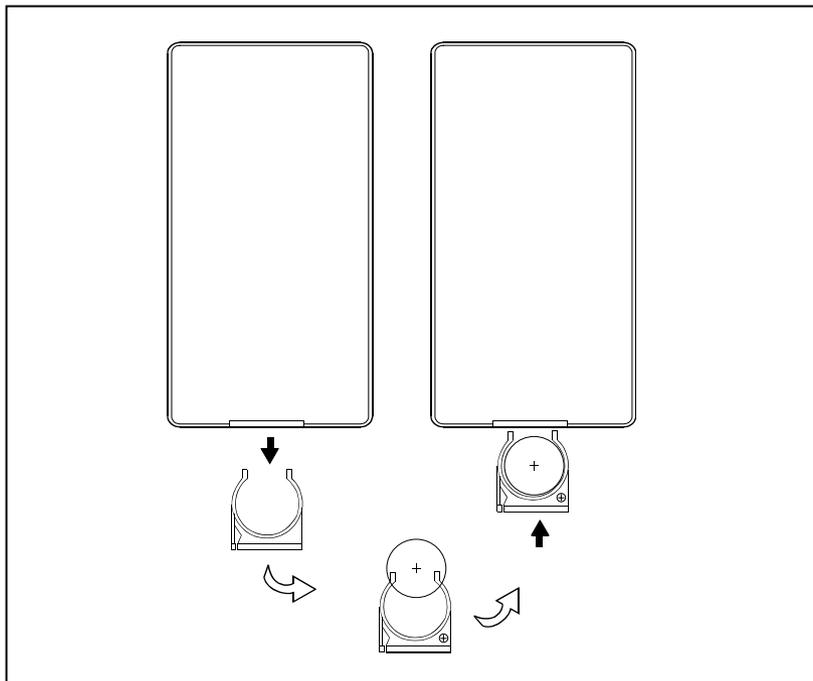
1. Referring to the drawing above, take the back cover off of the remote control and remove the empty battery receptacle.
