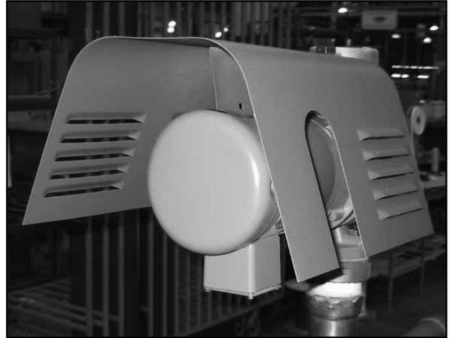
**Fig 17: Pump cover - angle view**
