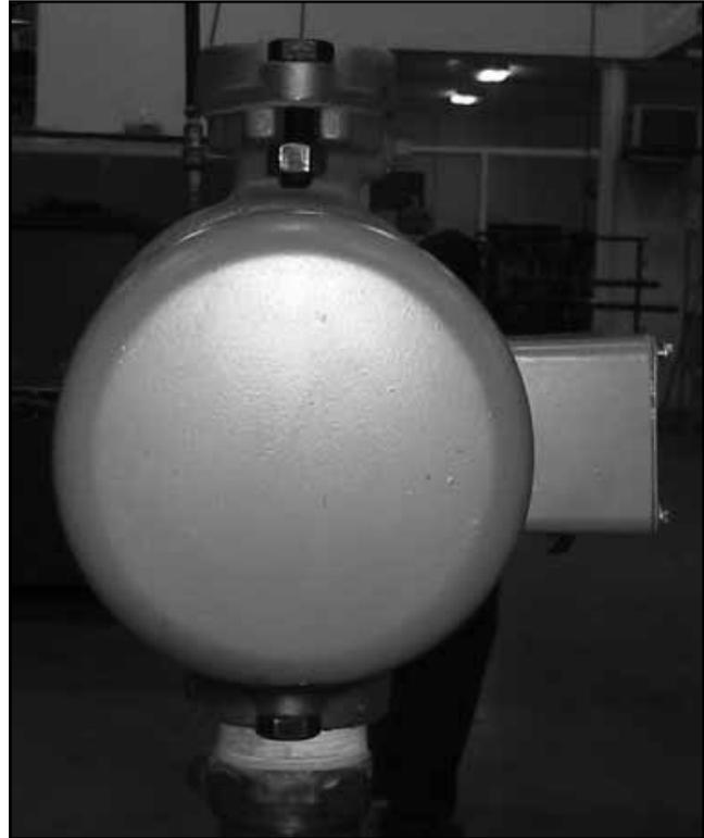
Fig. 13: Remove the pump body
