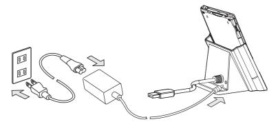
**Method 2.** Connect the supplied AC adapter and the Toshiba Pocket PC as shown in the figure below.
