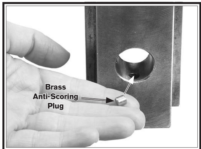
Figure 9. Slide block brass anti-scoring plug.
