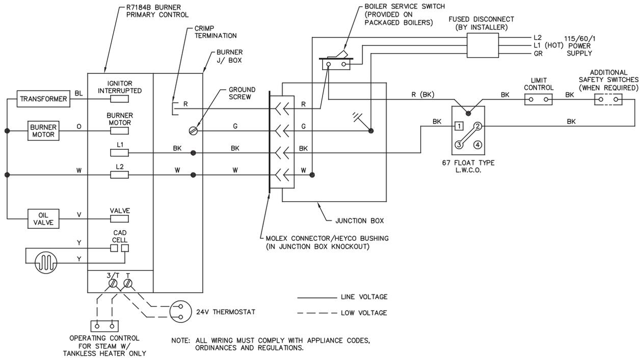
Figure 4.4: Steam with Float Low Water Cut-Off
