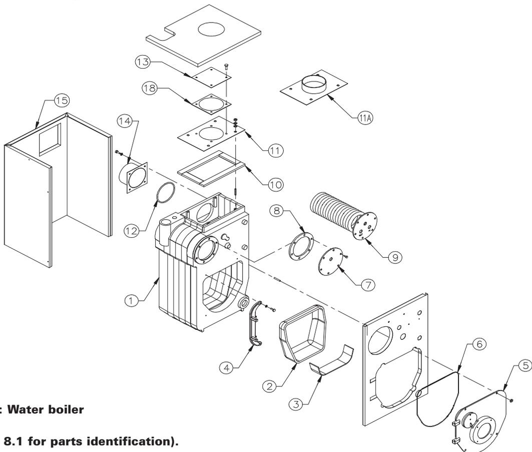
**Figure 2.2: Water boiler**
